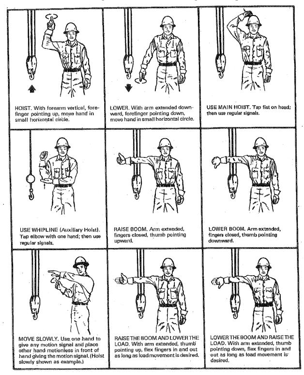
[Standard Hand Signals for Controlling Crane Operations]
