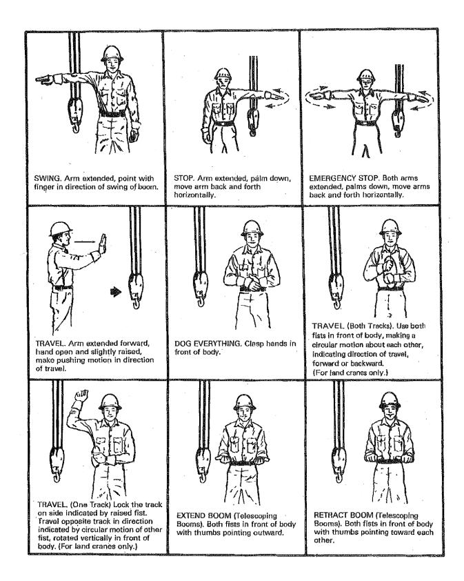
[Standard Hand Signals for Controlling Crane Operations]
